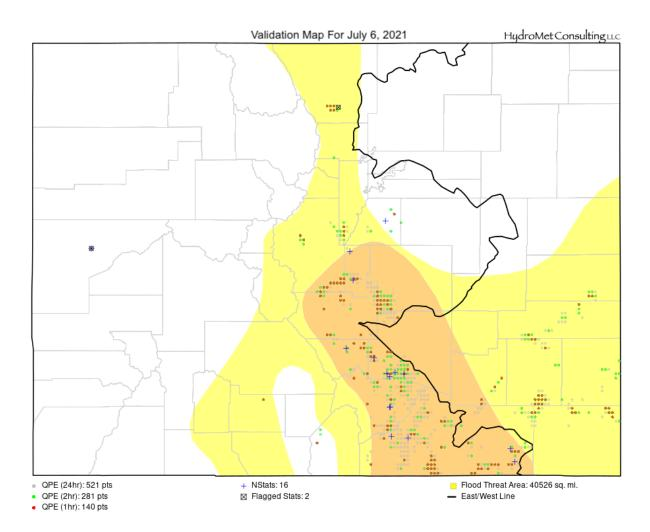
Figure 11: Example of daily verification map from July 6<sup>th</sup>, 2021 showing qualifying 1-hour, 2-hour and 24-hour MRMS grid points (gray), rain gauges (blue crosses) and threat area (yellow color fill).
